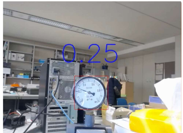
図 5. Automatic analog meter reading
