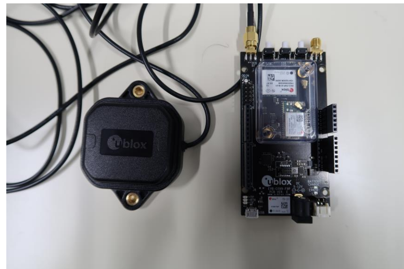
U-blox ZED F9P RTK-GNSS module
